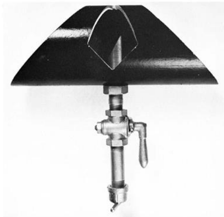
Figure 5 — In-line asphalt sampling device
