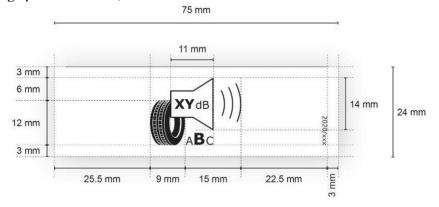
2.1.2. Format of the bottom part of the tyre label for tyres which satisfy the minimum snow grip index values set out in UNECE Regulation No 117:
