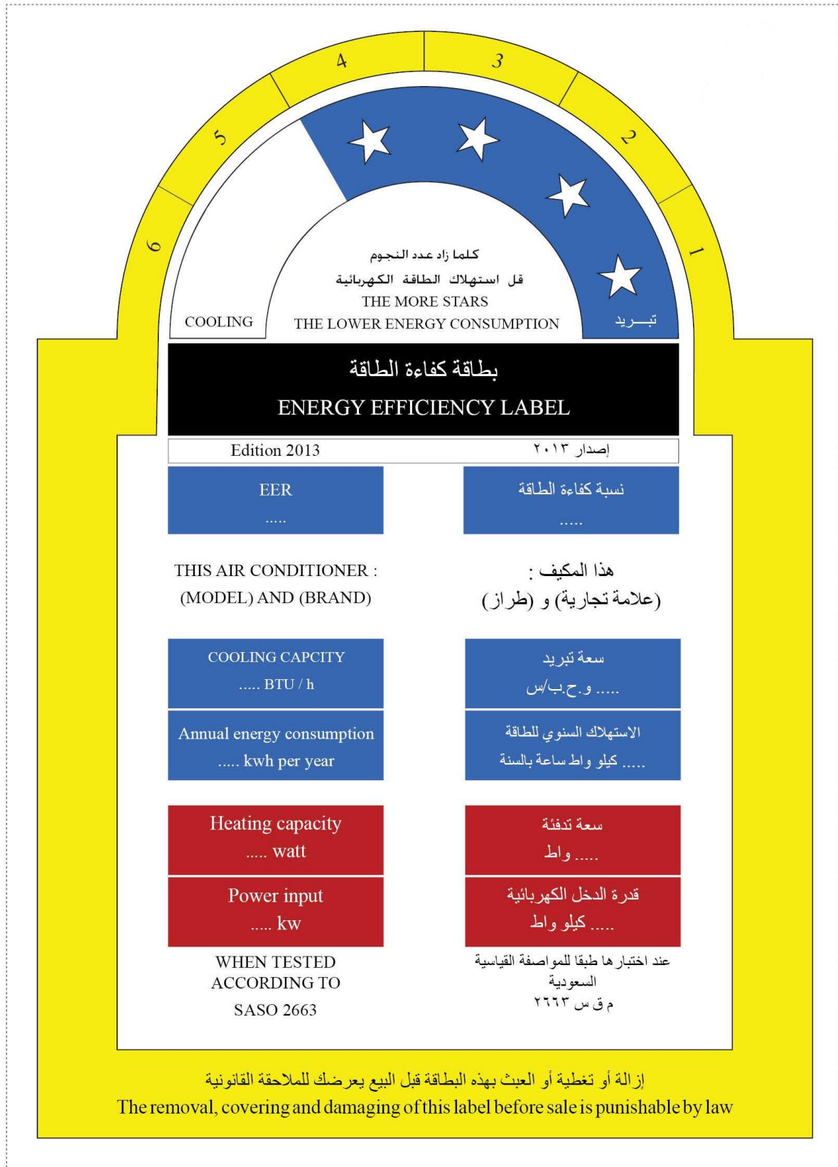
FIGURE 2: Example of label- Heating & Cooling Unit
