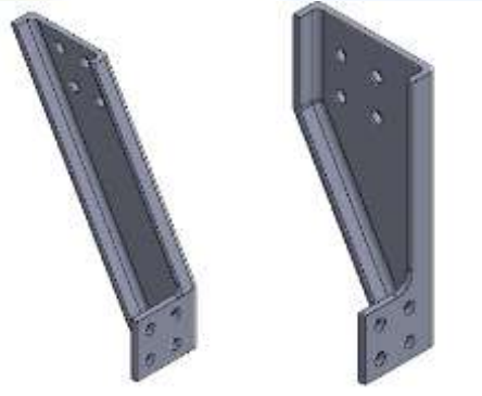
Figure 13: Sample of a carrier bridge used with (C-section beam) chassis truck or trailer
