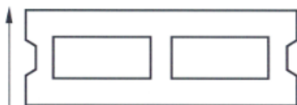
Figure B.31 — Lightweight concrete masonry units — Geometry 0,6/x
