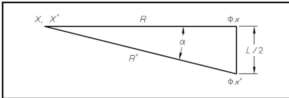
Figure D.3 — Configuration of lamp and photocell sensor
