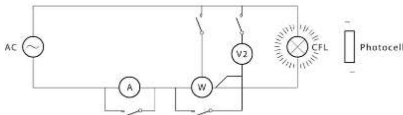
**FIGURE D1 – MEASUREMENT OF LUMINOUS FLUX**
