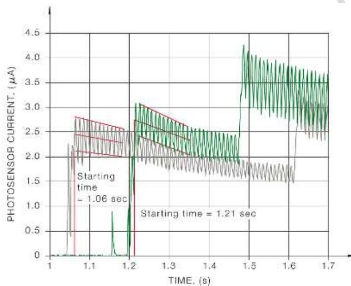
**FIGURE B2 – DIAGRAM FOR STARTING TIME (EXAMPLES 1 & 2)**
