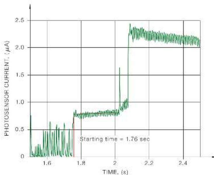
**FIGURE B3 – DIAGRAM FOR STARTING TIME (EXAMPLE 3)**
