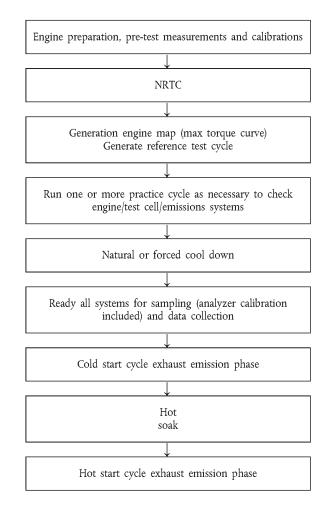
One or more practice cycles may be run as necessary to check engine, test cell and emissions systems before the measurement cycle.
