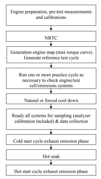
One or more practice cycles may be run as necessary to check engine, test cell and emissions systems before the measurement cycle.
