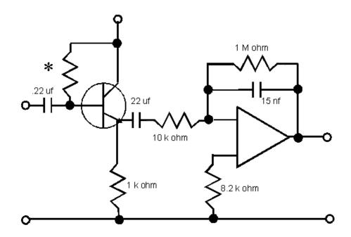
\* Select the value of this resistor to provide suitable collector current
